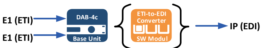
ETI-to-EDI converter with ETI Redundancy
